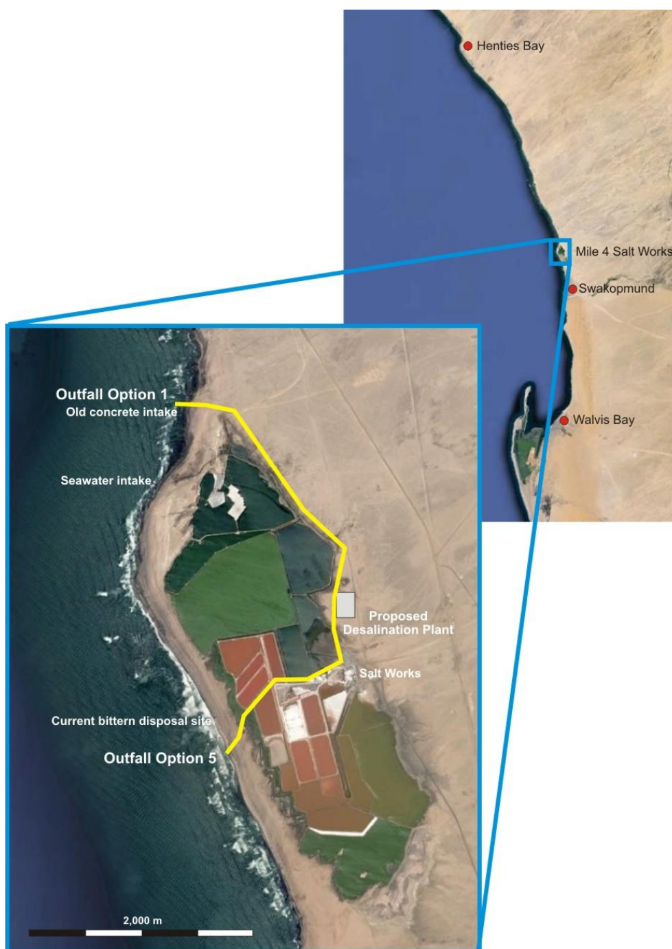
Figure 3: The location of the salt works and associated existing and proposed infrastructure in relation to the coastal zone between Walvis Bay and Henties Bay. The two alternative outfall options are shown (yellow lines).
