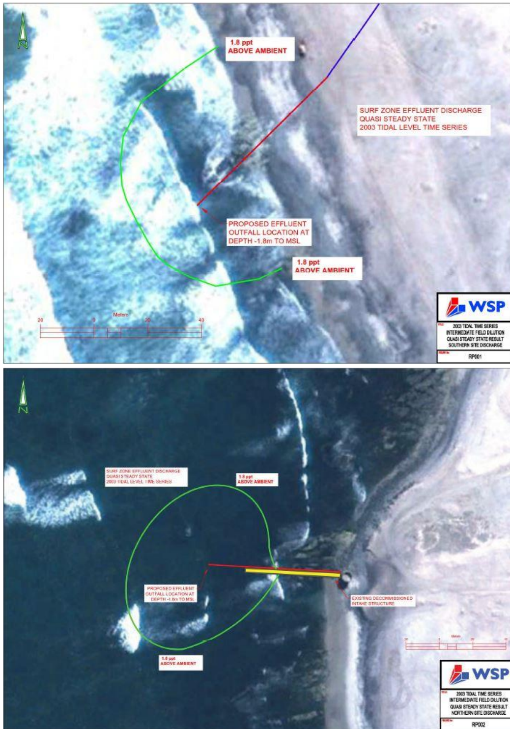
Figure 25: The diluted intermediate brine influence area for the southern (top) discharge location (Option 5) and the northern (bottom) discharge location (Option 1) (from WSP 2014b).
